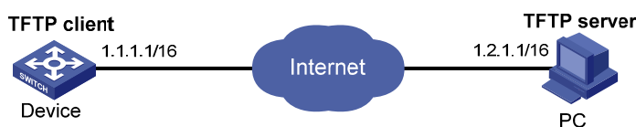
Figure 40 Smooth upgrading using the TFTP client function
